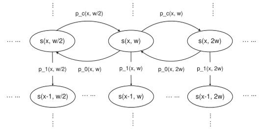
Fig. 3. State transitions of transient states in the Markov chain, where  $w$  is the contention window size. The number of tags,  $x$ , is decreased by 1 to identify each tag.
