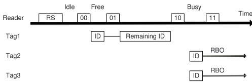
Fig. 1. RCSMA. The Reader broadcasts a Request Start command to start a tag identification task. In this task, the reader sends REQ command (four kinds of REQ, "00," "01," "10," and "11") to tell the channel condition (Idle, Busy, or Free) and divide time into slots. Each tag changes the contention probability in each slot. One tag will conduct Random BackOff (RBO) if collision occurs or transmit the remaining ID if the channel is free for transmission.
