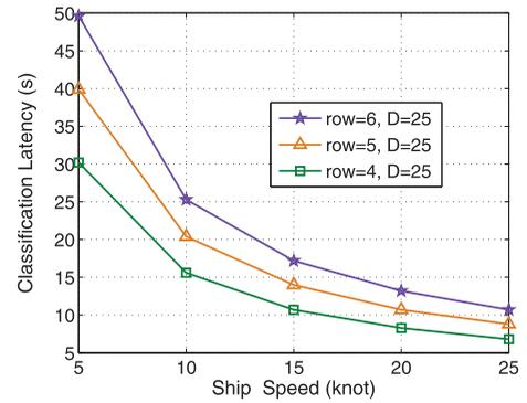
Fig. 9. Ship speed and classification latency.
