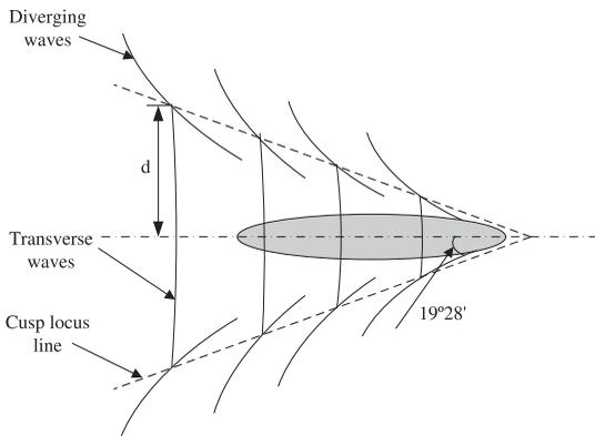
Fig. 2. Ship-generated wave model.
