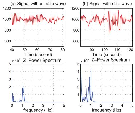
Fig. 3. Short-time Fourier transform. (a) Signal without ships and its spectrum. (b) Signal with ships and its spectrum.
