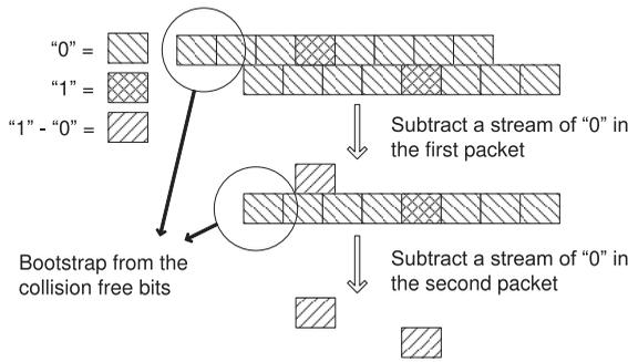
Fig. 1. Decoding two collided RNs. Only two bits left after subtracting all the known bits.
