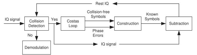
Fig. 4. The collision decoding diagram in RFID reader.
