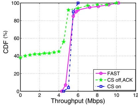
Fig. 9: Aggregate throughput for interfering node configuration.
