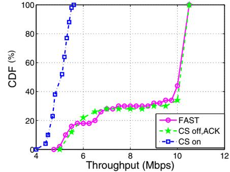
Fig. 10: Aggregate throughput for exposed node configuration.
