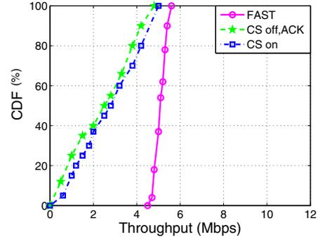
Fig. 8: Aggregate throughput for hidden node configuration.
