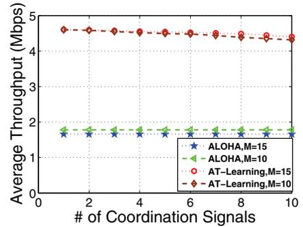
Fig. 8: Performance of AT-Learning and multi-channel Slotted-ALOHA with varying signal space  $C$  ( $M=10, 15$ ).
